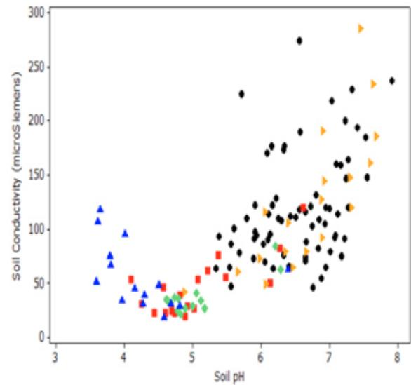
Fig. 4. The relationship between soil pH and soil conductivity. Soil types – black circles: calcareous; red squares: from sandstone; green diamonds: ultrabasic; blue triangles: from chert; orange arrow heads: alluvial.
